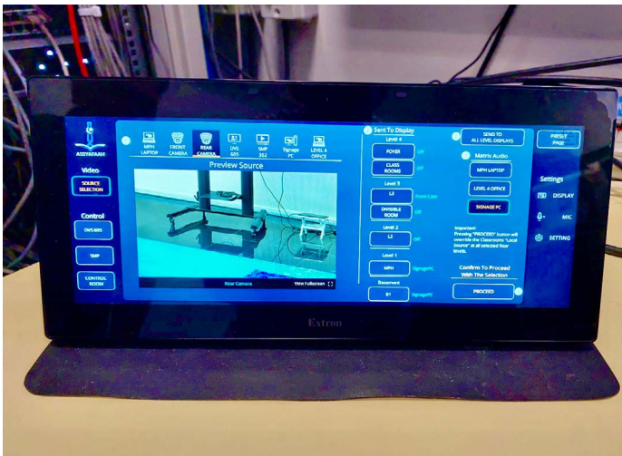
The Extron TLP Pro 1230WTG is a 12" Ultra-wide Tabletop TouchLink Pro Touchpanel.
